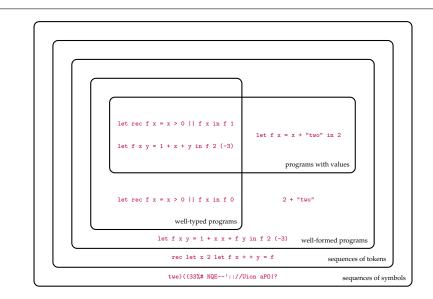
Figure 2.1: Visualization of nested classes of programs. In order to make the graphic simpler, the code examples are actually OCaml *expressions*, not programs.
